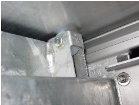
Support roller at the stern and part of the lateral support surface on the railing under the drive-up ramp
