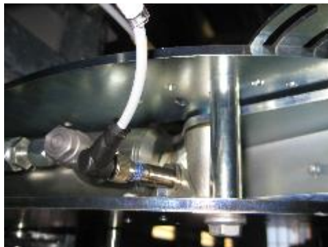
Sensor tilt scissors closed at the rear between the side cheeks of the tilt scissors
