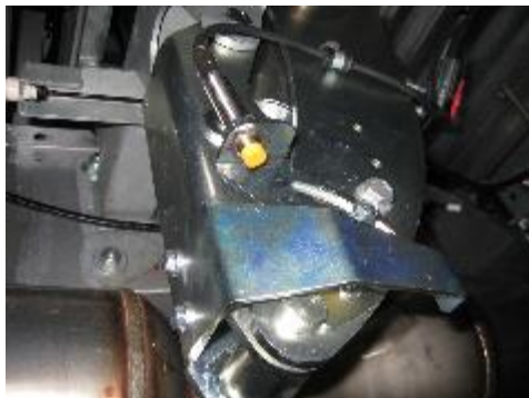
Sensor end position tipping shear attached to the side of the tipping shear
