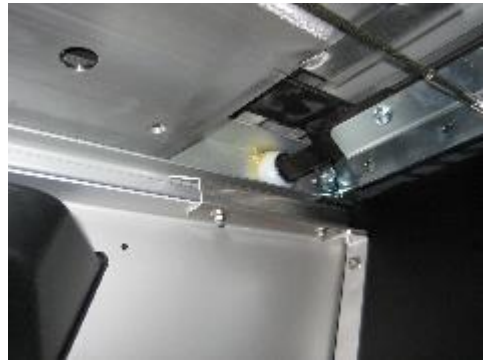
Guide roller at the end of the ramp
