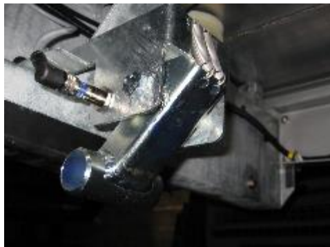
Tilt sensor at the rear lower end of the plateau
