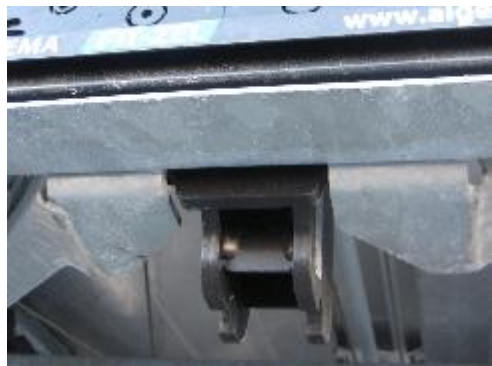
Mounting for ball bar at the bottom of the rear of the car transporter.
