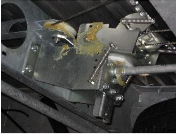
Center ramp actuation mechanism*
