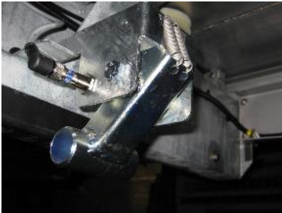
Tilt sensor with rocker switch at the lower rear end of the plateau
