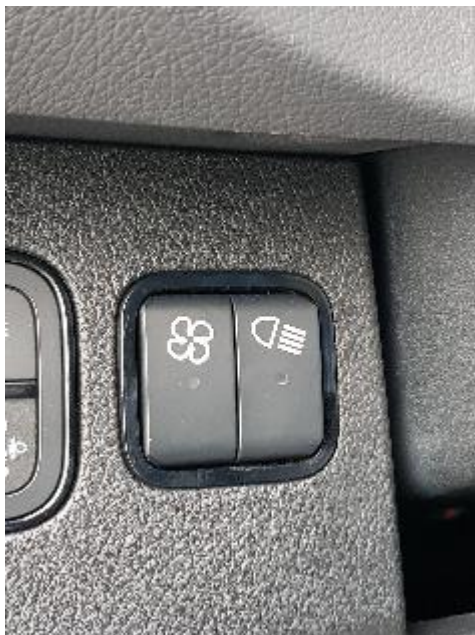
Switch left (case ventilation), right (coffer lighting)
