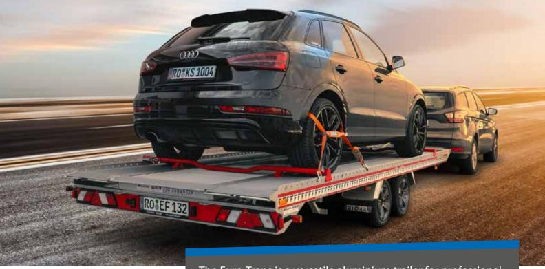
The Euro-Trans is a versatile aluminium trailer for professional vehicle transport. Up to 2.9 t payload make the Euro-Trans unique in its class. This is ensured by the particularly light all-aluminium construction with self-tipping mechanism.
